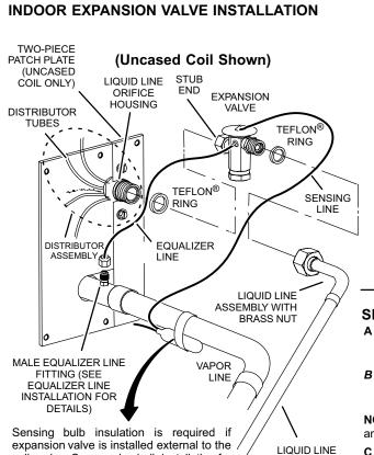
expansion valve is installed external to the LIQUID LINE coil casing. See sensing bulb installation for bulb positioning.
